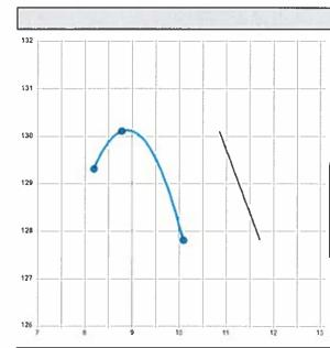
**Proctor ID:** P-03-std Maximum Dry Density (pcf): 130.1 8.9 Optimum Moisture (%): Specific Gravity: 2.70 Material on 3/4": Replaced 4163 Mold Mass (gr):
